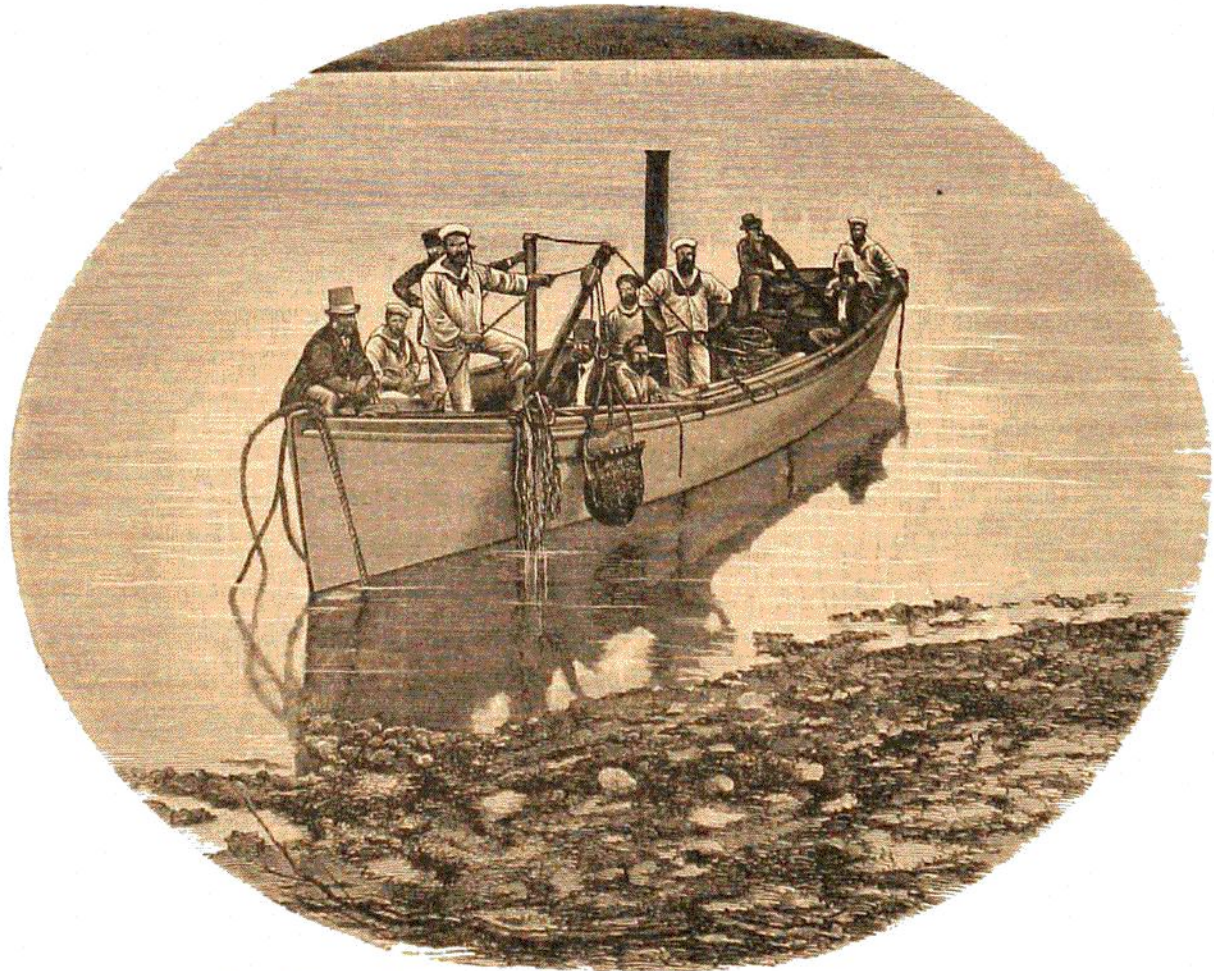
THE STEAM-PINNACE FITTED FOR DREDGING IN SHALLOW-WATER.
