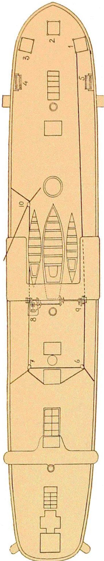
FIG. 1.—DECK ARRANGEMENT ON BOARD THE "CHALLENGER."
